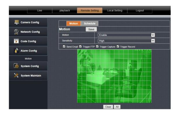
Motion detection is set to [Enable] to indicate that the motion detection function is in effect.
